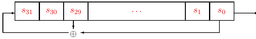
FIGURE 3. Linear feedback shift register: X^{32} + X^3 + 1
